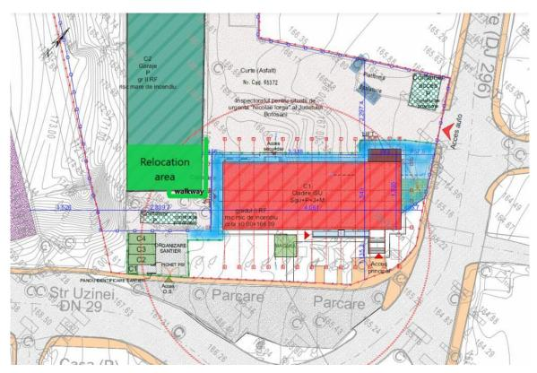
Fig. 5 Site organization; the area near the building that will be used for construction works is figured in blue
