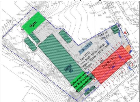
Figure 3 Designer drawing - The Land plot and the Buildings of BESI; the building that will be retrofitted is drawn in red.
